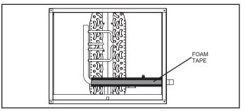
**FIGURE 1. Insulate Suction Line Inside Cabinet**
