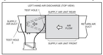
FIGURE 9. Static Pressure Test
