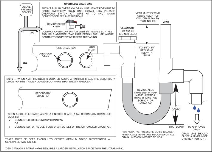
**FIGURE 8. Typical Main and Overflow Drain Installations**
