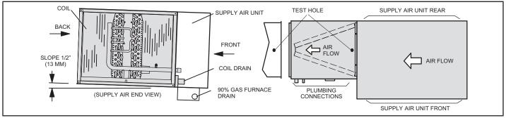
FIGURE 3. Left-Hand Air Discharge
