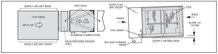
FIGURE 5. Right-Hand Air Discharge with Spacer
