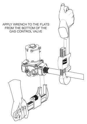
Figure 3: Proper Use of Wrench on Gas Control
