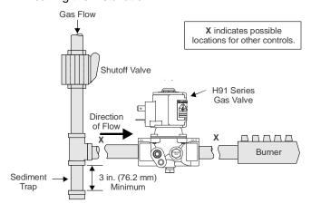
Figure 8: Typical H91 Installation
